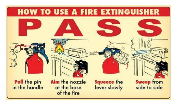
Note: When using fire extinguisher, pay attention to the direction of the wind. Always extinguish with the direction of the wind.
